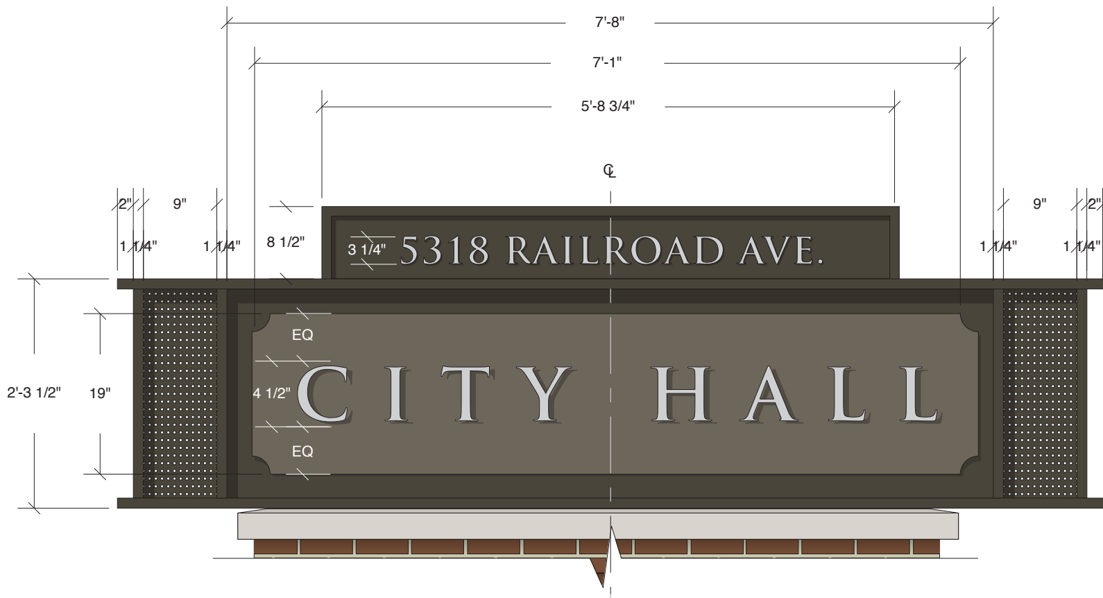
1 BUILDING ID - ELEVATION DETAIL SCALE: 1/2" = 1'-0"
