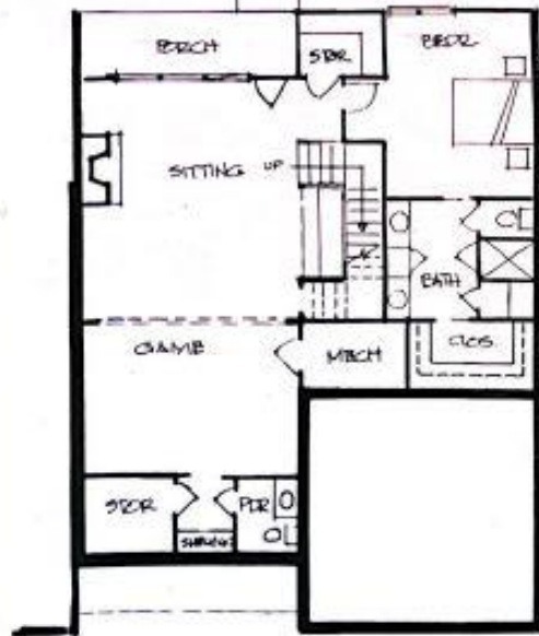
BASEMENT FLOOR PLAN (BASEMENT UNFINISHED-PLAN SHOWN AS OPTIONAL)
