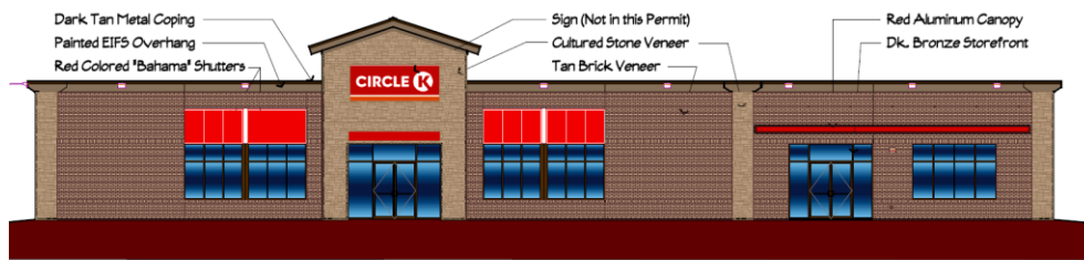
① FRONT ELEVATION OPTION 1/8" = 1'-0" 0 4 8 12 SCALE IN FEET
